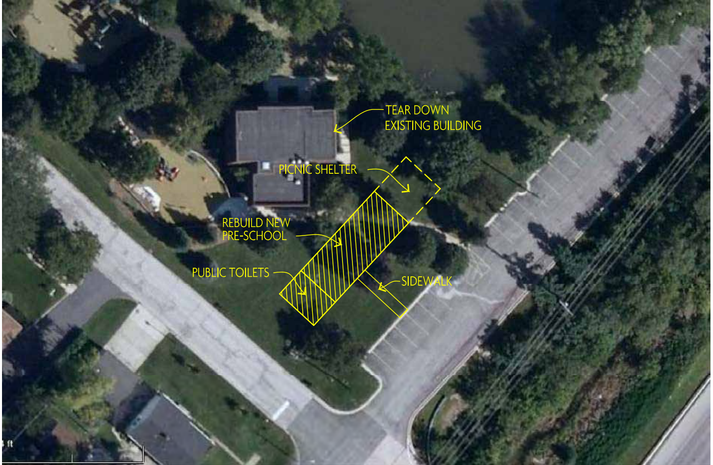
Solution 2: Tear Down & Rebuild New Simple Building to Serve One (1) Preschool Class Eldridge Park Recreation Building
