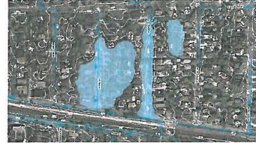
Figure 6. Pine Street XP-SWMM Simulated Inundation Area - July 2010 Storm Event
