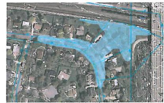
Figure 20. Brynhaven XP-SWMM Simulated Inundation Area - July 2010 Storm Event
