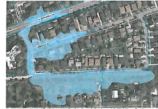
Figure 23. Yorkfield XP-SWMM Simulated Inundation Area - July 2010 Storm Event
