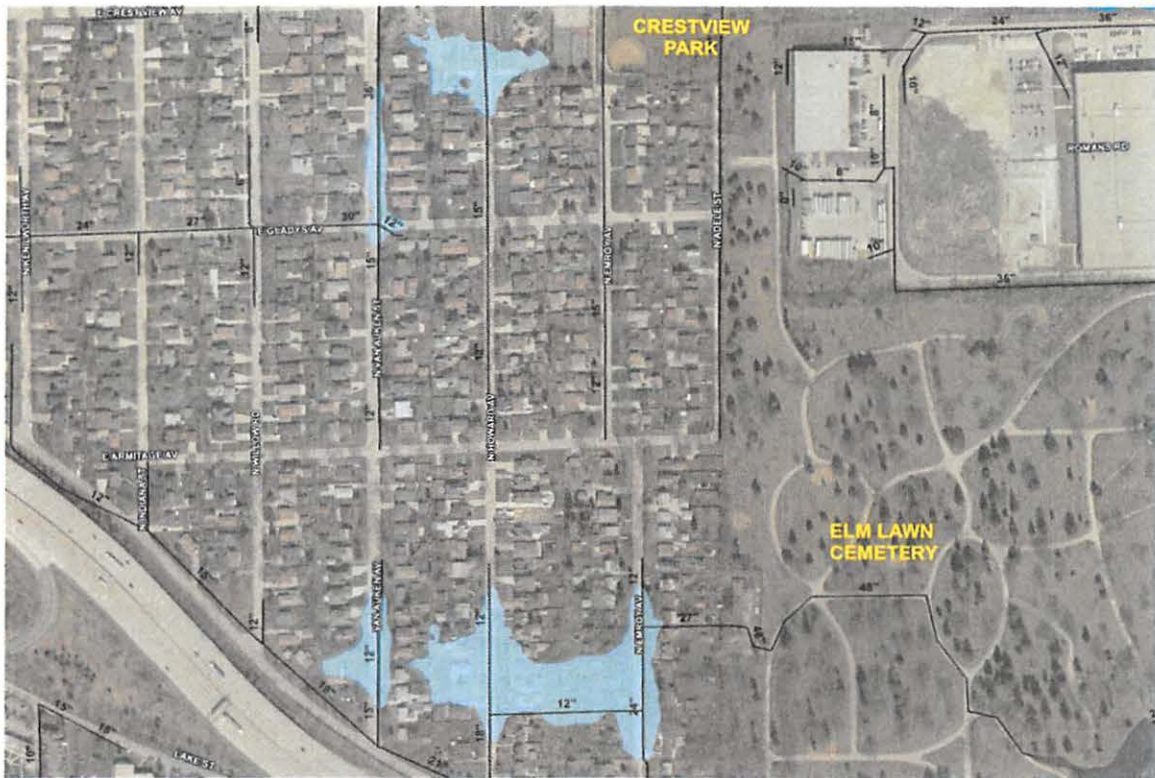
Figure 9. XP-SWMM Simulated Inundation Area – April 2013 Storm Event
