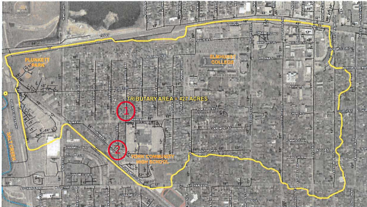
Figure 6. Overall Drainage Exhibit for the Collegeview Study Area
