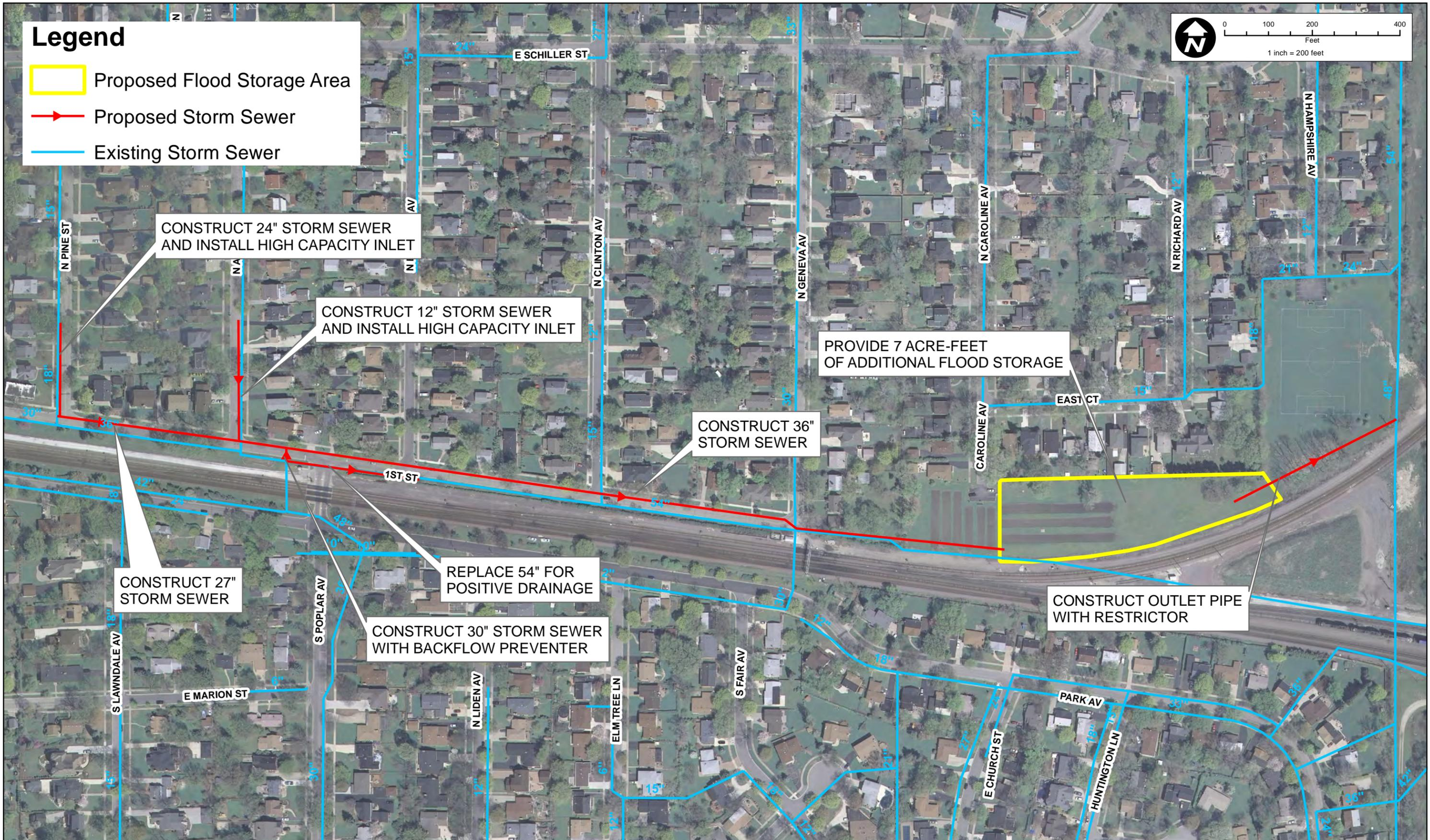
CONSTRUCT 24" STORM SEWER AND INSTALL HIGH CAPACITY INLET
