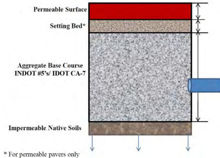
**Figure 24. Typical Pervious Pavement Cross-Section**
