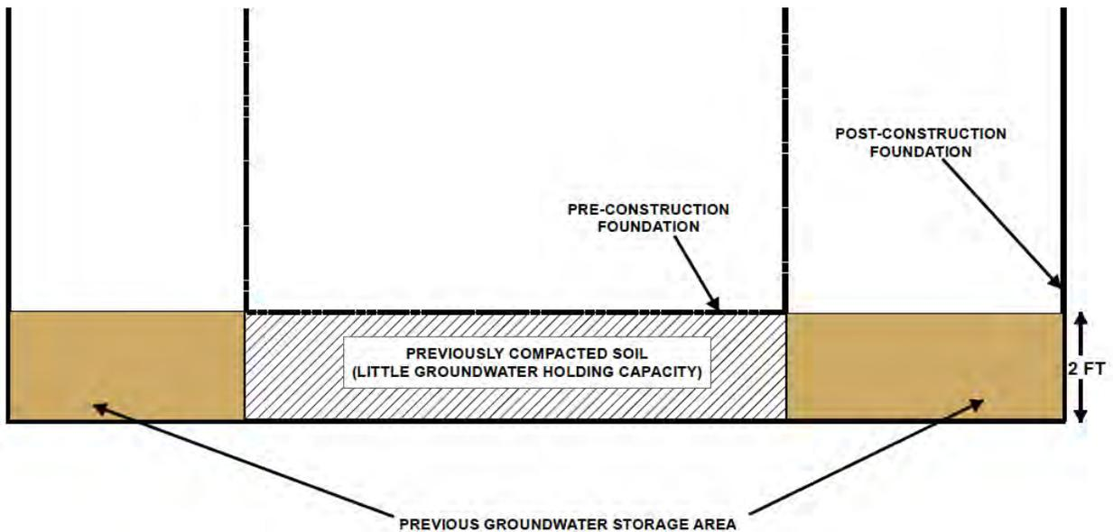
**Figure 27. Groundwater Displaced by Deeper Basement**
