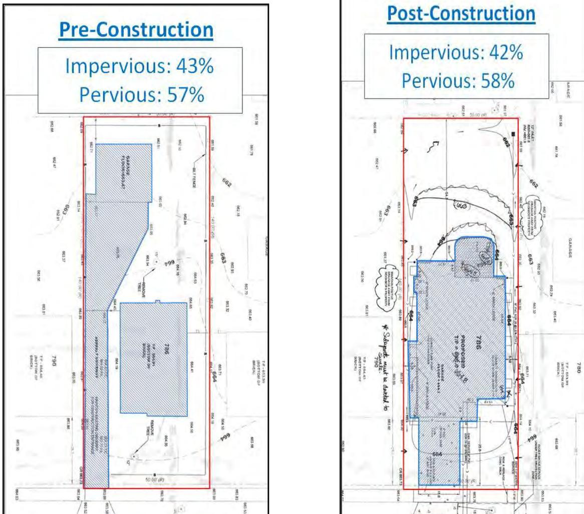
Figure 26. Pre- and Post-Construction Site Plan for 786 Hillside Avenue
