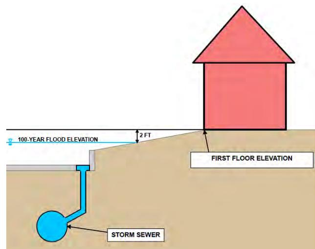
Figure 28. Flood Protection System
